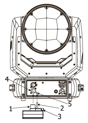
Push in the 5-pin XLR plug (1) into 5-pin XLR sockit (4) and simultaneously locating pin (2) into hole (5) in the fixture. In this way the wireless DMX module is connected with the fixture.
