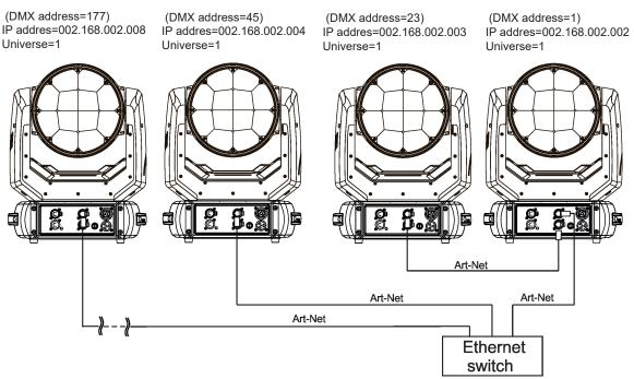
An advised PC setting: IP address: 002.xxx.xxx.xxx (Different from fixtures IP addresses) NET mask: 255.0.0.0
