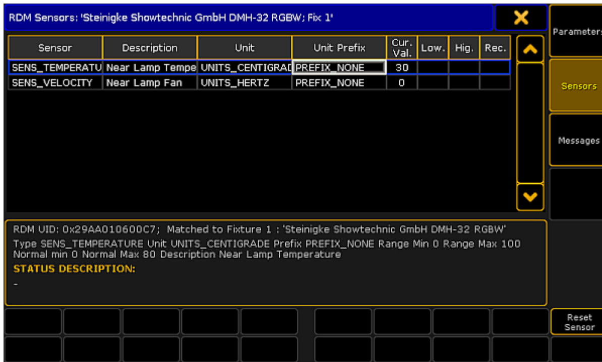
RDM sensors window
